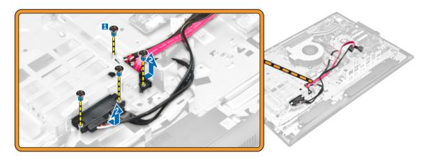
5. Disconnect all the cables that are connected to the system board.
