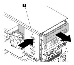
Figure 23. Removing the optical drive
