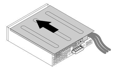
Figure 39. Reinstalling the flex module cover
