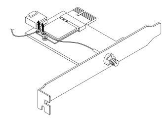
Figure 85. Disconnecting the Wi-Fi antenna cables
