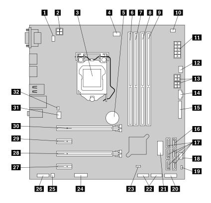
Figure 4. Parts on the system board
