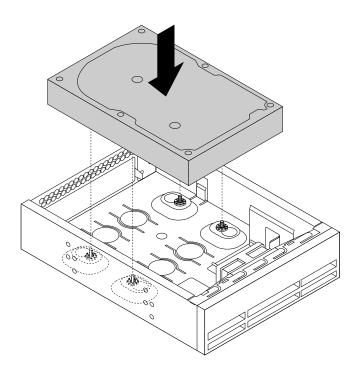
Figure 72. Installing the tertiary hard disk drive
