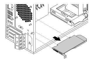
Figure 13. Removing a PCI card
