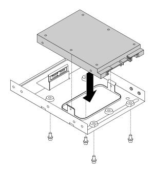
Figure 60. Installing the solid-state drive into the storage converter
