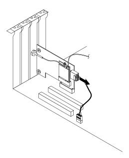
Figure 82. Disconnecting the Bluetooth cable
