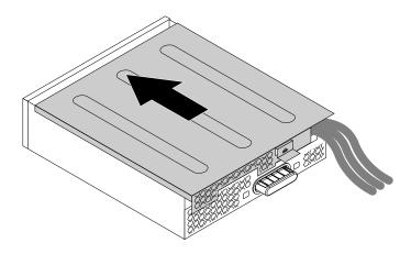
Figure 33. Reinstalling the flex module cover
