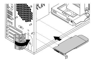
Figure 15. Installing a PCI card
