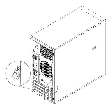
Figure 7. Installing a padlock
