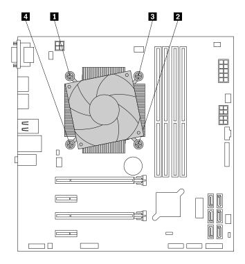
Figure 59. Removing the heat sink and fan assembly
