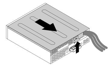
Figure 40. Removing the flex module cover
