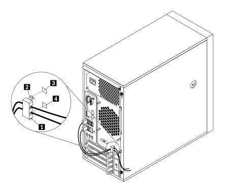
Figure 9. Installing a cable lock
