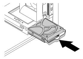
Figure 71. Installing the secondary hard disk drive
