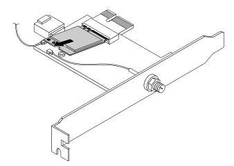
Figure 87. Removing the Wi-Fi card module
