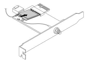
Figure 88. Installing the Wi-Fi card module
