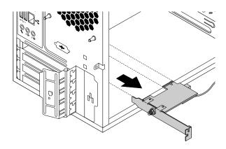
Figure 84. Removing the Wi-Fi adapter card
