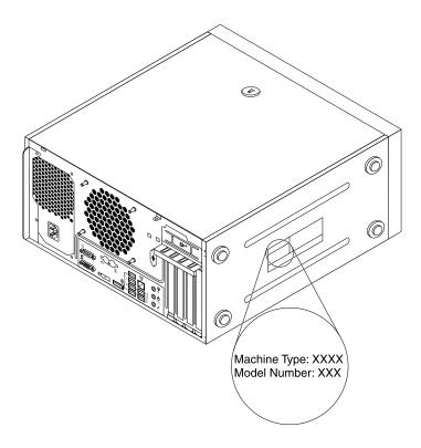
Figure 6. Machine type and model label
