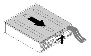
Figure 34. Removing the flex module cover
