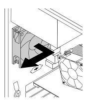
Figure 80. Removing the rear fan assembly
