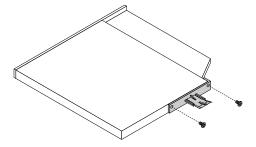
Figure 30. Removing the plastic clip from the slim optical drive
