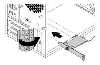
Figure 91. Installing the Wi-Fi adapter card
