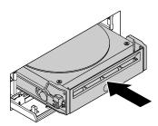
Figure 48. Installing the hard-disk-drive bracket
