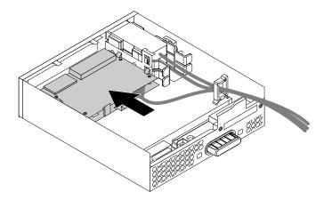
Figure 38. Installing the card reader in the flex module
