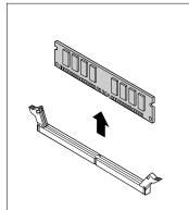
Figure 19. Removing a memory module
