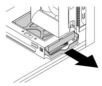
Figure 69. Removing the secondary hard disk drive
