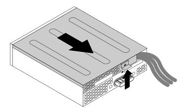
Figure 27. Removing the flex module cover
