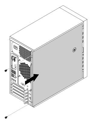
Figure 92. Reinstalling the computer cover
