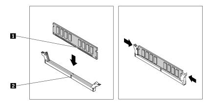
Figure 21. Installing a memory module
