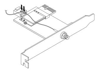
Figure 90. Installing the Wi-Fi antenna cables
