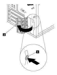
Figure 12. Opening the PCI card latch
