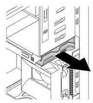
Figure 66. Removing the primary hard disk drive
