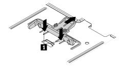
Figure 28. Removing the plastic clip with the two screws
