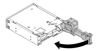
Figure 55. Pivoting the rear cover inward
