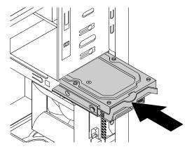
Figure 68. Installing the primary hard disk drive
