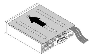
Figure 43. Reinstalling the flex module cover
