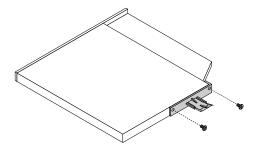
Figure 31. Installing the plastic clip to the slim optical drive
