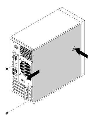
Figure 10. Removing the computer cover
