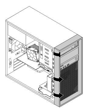
Figure 11. Removing the front bezel
