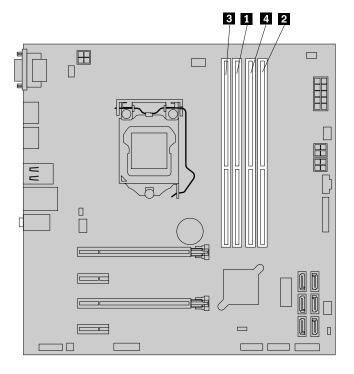
Figure 18. Memory module installation-order
