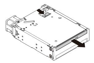
Figure 49. Removing the slim optical drive from the enclosure
