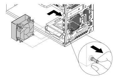
Figure 79. Installing the front fan assembly
