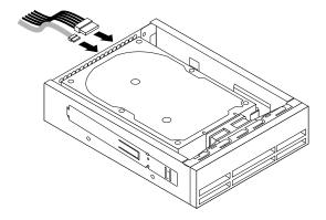
Figure 77. Connecting the hard disk drive or solid-state drive
