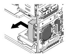
Figure 78. Removing the front fan assembly
