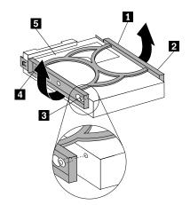
Figure 70. Installing the hard disk drive into the bracket
