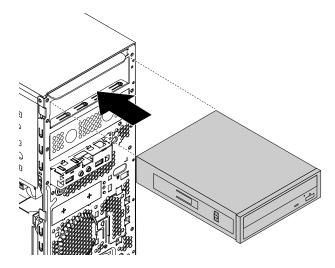
Figure 25. Installing the optical drive
