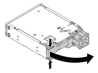
Figure 51. Opening the enclosure from the rear
