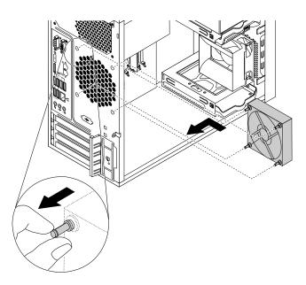
Figure 81. Installing the rear fan assembly
