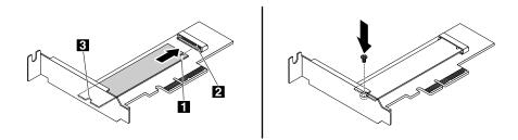
Figure 17. Installing the M.2 solid-state drive
