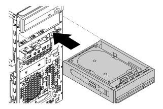
Figure 76. Installing the optical drive bracket
