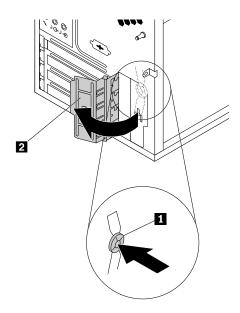
Figure 83. Opening the PCI card latch
