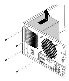
Figure 58. Removing the screws for the power supply assembly
