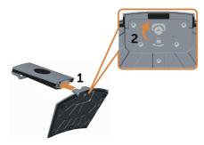
Attach the stand assembly to the monitor.
