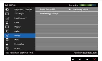
Power Button LED Allows you to set the state of the power light to save energy.
