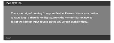
If either VGA or HDMI (MHL) 1 or HDMI (MHL) 2 input is selected and the corresponding cable is not connected, a floating dialog box as shown below appears.
